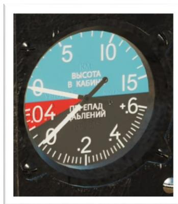
**UVPD-15 COCKPIT ALTIMETER & DIFFERENTIAL PRESSURE INDICATOR**
