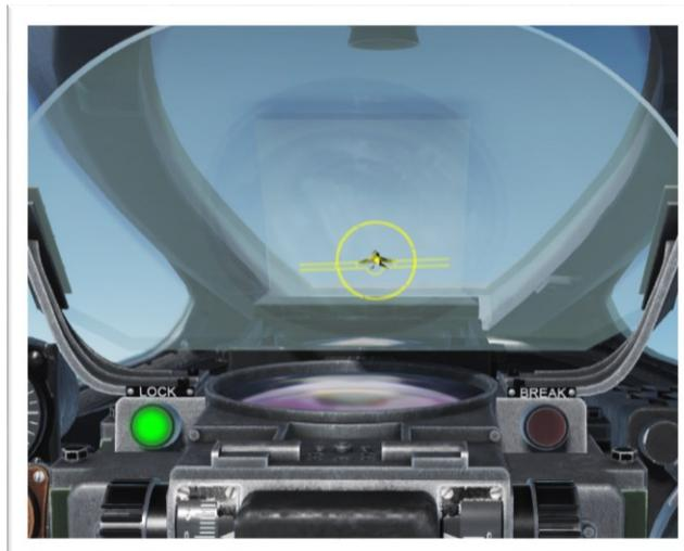
5. If you hold you Fire to get close on the Target Aircraft, keep in mind that, like the Radar, the Sight also displays a Proximity Alert, represented by the Red Break Lamp. As the distance to the Aircraft approaches 300 meters, the Break Lamp will illuminate.
