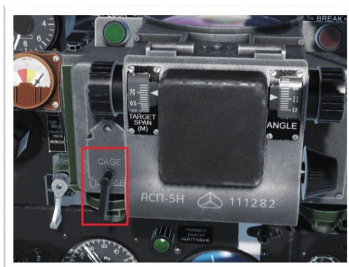
4. Having selected the Target Wing Span, change the Aiming Reticule Distance by rotating the Throttle Handle backwards and forwards, check the change in the Diameter of the Outer Circle.
