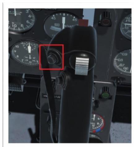
This Button is an electrical Caging, Centering the Gunsight Reticle when pressed. This way, the Pilot can introduce the correct Distance into the Sight during intense maneuvering while the Lead Angle Calculations for the selected Distance are still made. When the button is released, the Reticle returns to the Calculated Impact Point Position (CIIP).
