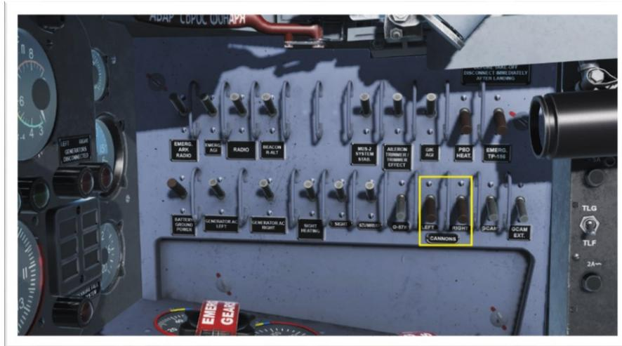
2. Press the Cannon Reload Buttons on the Upper LH Side panel for more than 2 seconds per Button.
