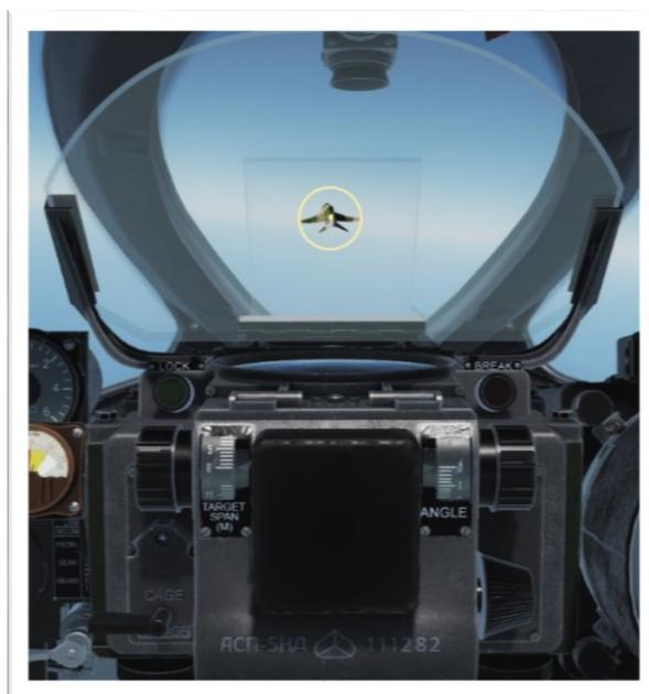
During this process, as the Gunsight Gyros are Uncaged, it may be possible that during high G maneuvers, the reticle moves too far down, disappearing from the Sight Field of View. While this may not be an issue at Short Range, because Bullet deflection is not relevant, it may prevent effective engagement of Targets at Medium to Far Distances as in this case it will be impossible to introduce the correct Distance for a good Aiming Solution.
