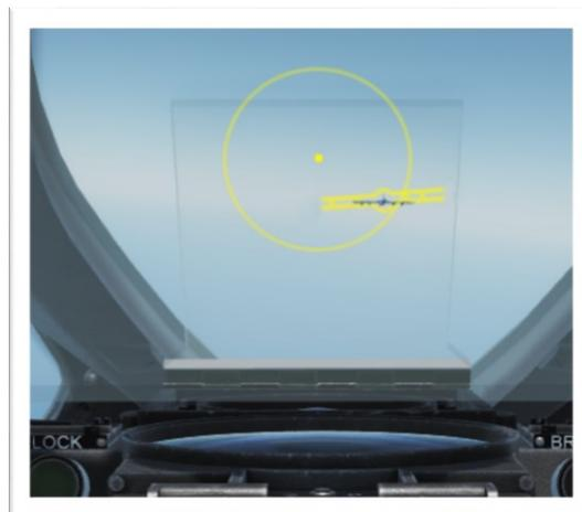
6. As the Distance to Target approaches 300 meters, the Red Break lamp will illuminate, instructing the Pilot to Turn away and leave the attack run to avoid a collision. After 3 seconds the Lock will be dropped, as well as all Aiming Solution.
