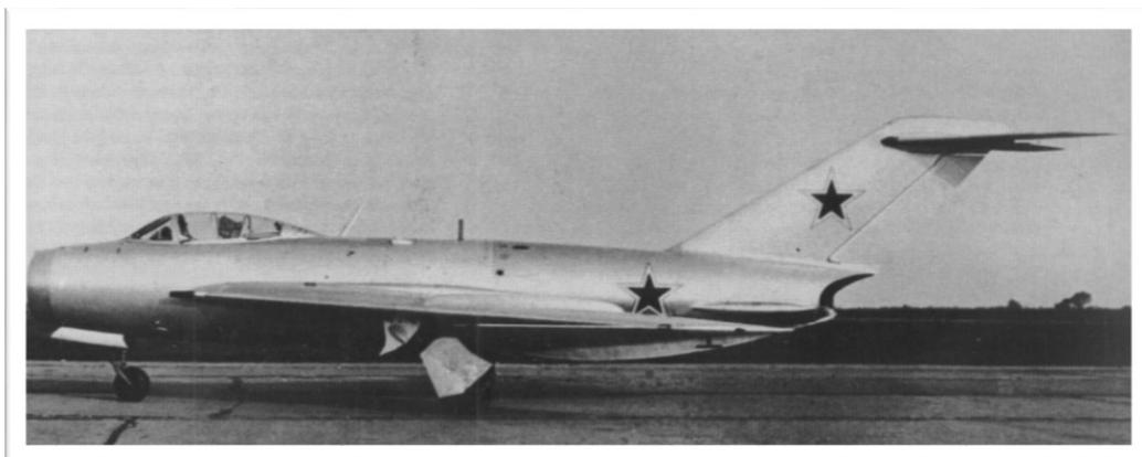
**The SM-2 prototype was a MiG-17F airframe modified to use two AM-5 engines, with an enlarged fuselage and a new wing design**
