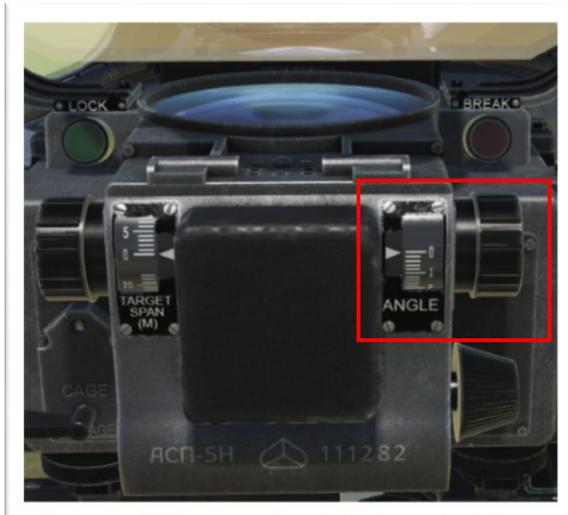
5. The same as Cannon or Rockets use, select a Target Span (if between 7-70 meters) and desired Distance for Bombing (depending on the target, the best bombing distance is from 1,500 to 2,000 meters).
