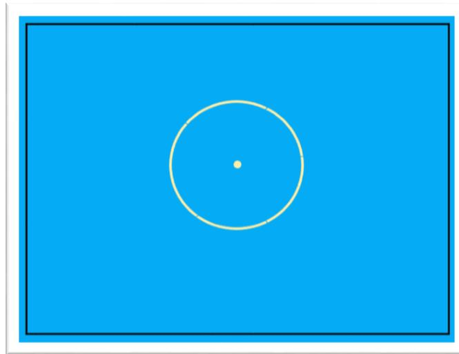
When in Caged Mode, the Sight will maintain the indication centered at the correct Aiming Point based on Distance for a Static Aircraft. When the Distance is changed in the Caged Mode, by rotating the Throttle Grip, the Reticle will move up or down to compensate for bullet drop.
