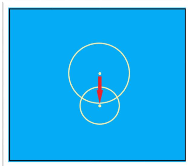
The Image above is an example of the Sight Indication when increasing the Distance to Target. The Larger Circle is the initial position and the Smaller Circle is the final position. Note the Diameter Decreases and the Cannon Aiming point moves Down, compensating for bullet drop.
