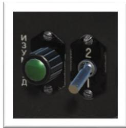
2. This turns off the AR-18-1 Search Antenna of the Radar and any Target within 1,200 meters of the Aircraft will be Locked. The Radar will then work identically to a Radio Range-Finder, like the one installed in the MiG-19S.
