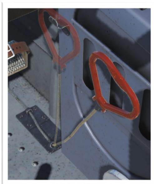
**LANDING GEAR EMERGENCY DEPLOYMENT HANDLE**
