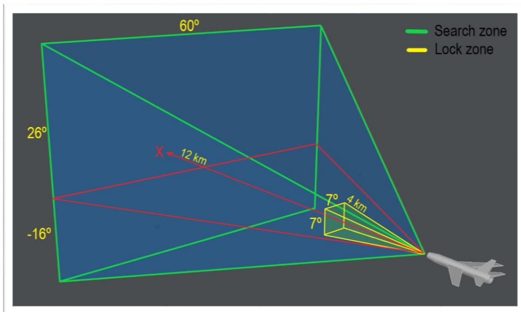
The RP-5 is heavily affected by Ground returns at Low Altitude, making it impossible to use at Altitudes below 2,000 meters. The Radar has an Altitude Mode Switch, on the Main Instrument Panel, which disconnects the Search Antenna and reduces the Track Antenna Range from 4,000 to 1,200 meters. This allows for Automatic Aiming Solutions from 2,000 meters down to 1,000 meters in Daylight Conditions. This transforms the RP-5 into a Radio-Rangefinder.
