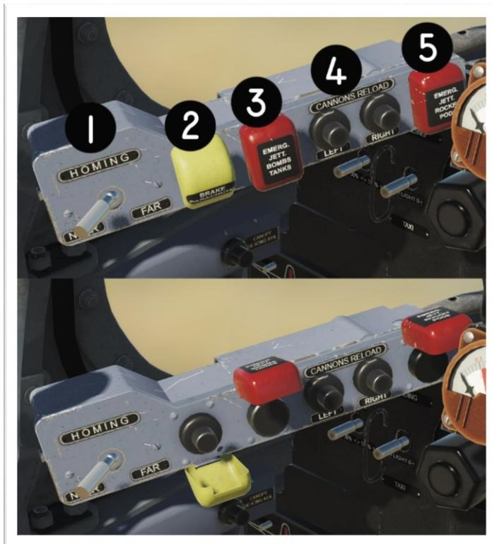
1. Homing Switch. It switches the ARK-5P NDB Receiver to the FAR or NEAR Pre-Set Beacon/Freq Selector.
