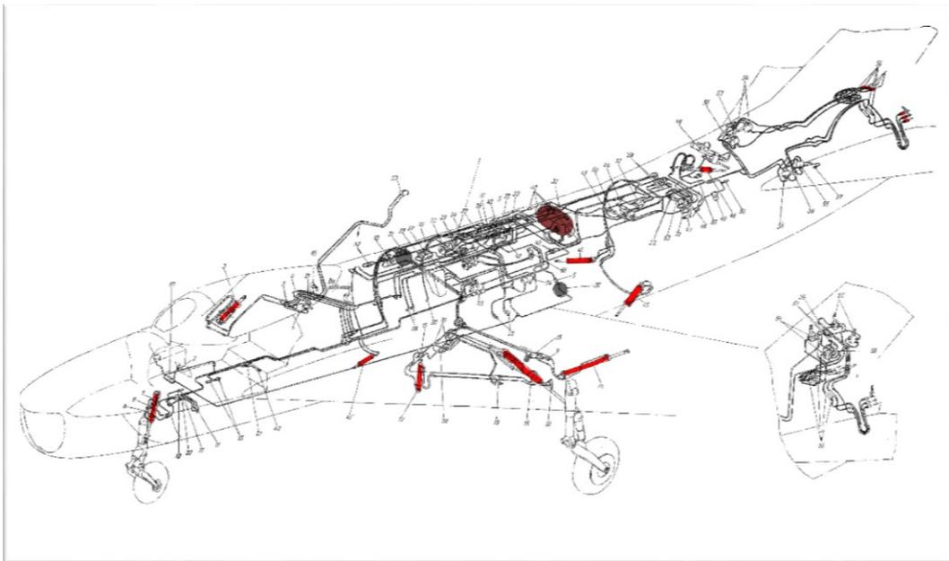
Both systems are independent and operate all the Hydraulic consumers by separate chambers and Check Valves. So, in case any of them fails, the other will take over the functions.
