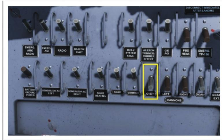
2. On the ASP-5N Control Panel, put the Armament Mode Selector in Rocket Pods (P.C).
